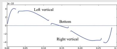
With longer wires, the nearly constant gradient of rings of surface charge is even more apparent.
