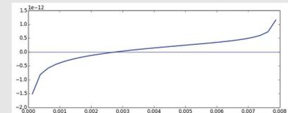
A graph of the ring charge along the polarized block of metal shown above. Along much of the block there is a nearly constant gradient of surface charge, with charge buildup on the ends.
