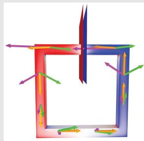
For this simple circuit, orange arrows represent the net field along the centerline of the wire, magenta arrows represent the field contributed by the capacitor, and green arrows represent the field contributed by all of the surface charges.
