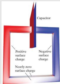
A simple circuit shows a roughly constant gradient of surface charge along the wires.
