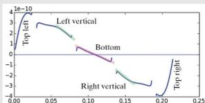
A graph of the surface charge density ( $C/m^2$ ) along the wire in the simple circuit shown above, averaged over a (square) ring drawn around the wire, as shown below; to average out transverse polarization that does not affect circuit behaviour. There is a roughly constant gradient of rings of surface charge along the wire. The graph omits the complications at the corners.
