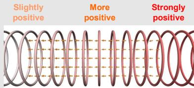
A constant gradient of charge on a line of rings produces a remarkably uniform electric field inside the rings, like the field inside circuit wires.
