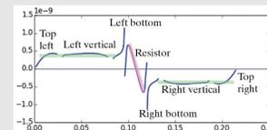
A thin section of wire acts as a resistor. Charge buildup at the ends of the thin wire, visible in the graph, leads to a negligible gradient of surface charge along the thick wire and a very large gradient of surface charge along the thin wire, producing the large field necessary to drive the same amount of current through the thin wire as flows through the thick wire.
